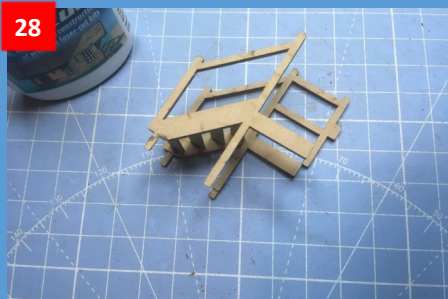
28 Trim off any step that is protruding and glue side rail right (34) as shown
