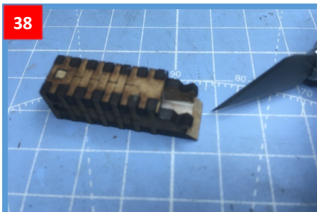
38 Once dry, trim the inside of the chimney front (43) to match the angle of the sides
