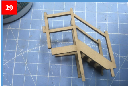
29 Trim off any step that is protruding and glue side rail left (35) as shown
