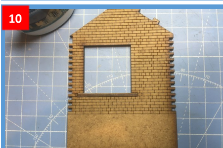
10 Glue windowsill (17) to the right wall (13) ensuring it is flush at the back
