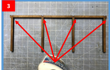
3 Prepare and glue parts 3 & 4 together as shown ensuring the engraved lines are facing out
