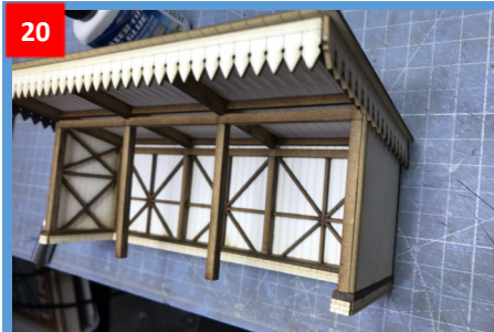
20 Glue dagger boards as shown and leave to dry
