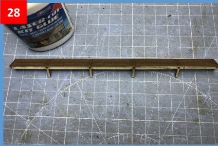
28 Glue bench planking, part 32 to the bench frame an leave to dry
