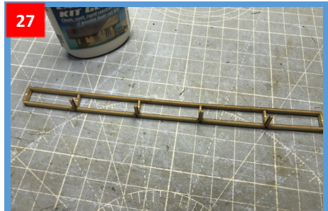
27 Glue the front bench frame, part 29, to the rear frame assembly and allow to dry
