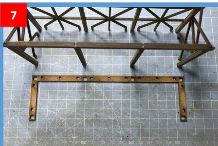
7 Prepare part 7, a light sanding of the frame "legs" may be required for a good fit
