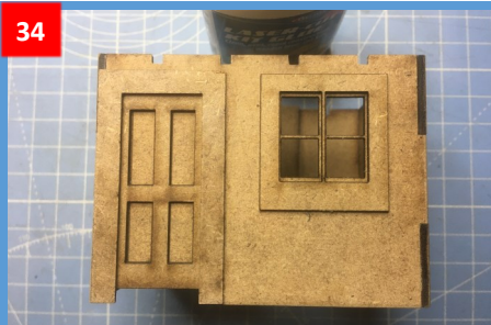
34 Glue the outer frame (32) to the face of the inner wall ensuring it is square and equal
