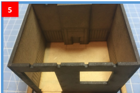
5 With the walls positioned on the base, glue the fireplace using the engraved lines as a guide
