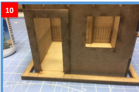
10 Glue the door frame (13) into position on the outside of the inner wall .....
